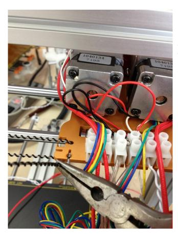
If you are having trouble getting it tight enough you might use a pair of pliers to pull the synchromesh up out of the second hole. Tighten down X carriage motor mount when done. The X-carriage synchromesh does not have an adjuster screw the way the Y-carriage one does; swinging the motor mount accomplishes the same thing.
