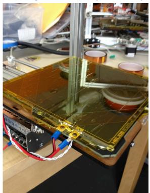
Take the kapton tape (yellowish clear tape) and the sheet of glass and tape the glass down on top of the heated platform. Cover the entire platform without gaps or overlaps. This is the surface you will use for printing most plastics. (Nylon requires a different platform surface.)
