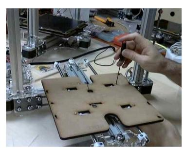
mount to the clear platform support you just put on. Be sure the "Front" label is on the side away from the azteeg board support and be sure they are very tight. Check that the assembly slides smoothly.
