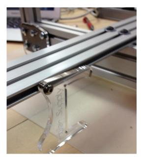
Attach the big "Power Supply" mount to the Y center beam. You will adjust it at the very end of the process, but just attach it for now and we will move it.
