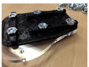
Lay out the four bottom feet/corner clear brackets (see picture below) thinking ahead about the through the orientation of all four. (Unfortunately it is easy to flip the acrylic.) Take the clear acrylic piece and the black plastic piece, and put the M5 screws on the outside of each piece, screwing through the black plastic.
