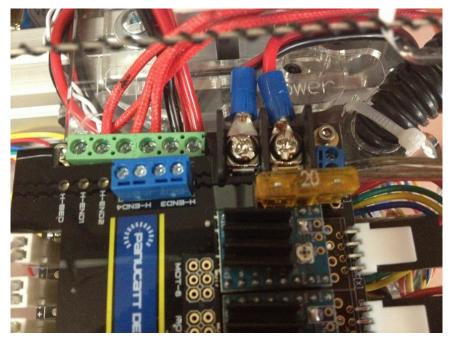
Strip the ends of the extruder heater wires and insert them into the "H-end" pairs on the Azteeg board (if you only have one extruder, just use #1). Since these wires are not quite long enough to go down and through the connector board mount, you should separate them out a bit higher than the end of the cable conduit and run them across the TOP of the connector board mount.
