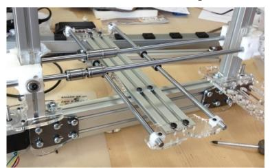
the bottom of their Z travel so that the holes line up. You might have to ream out the holes a little to get the rods in.
