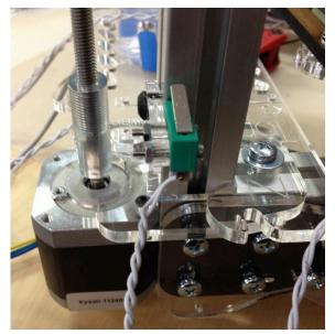
Now assemble the z axis stop. It will attach to the Z motor vertical support on the Azteeg board side below the X motor. Screw in and fasten with nuts. Be sure this stop is stiff and well-mounted since if it is not your first layer may have issues.
