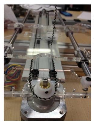
Add the zip ties on the other side. Tighten down the platform by pulling on the zip ties and make it tight. Once they are all tight trim off the excess. Do not trim the synchromesh; you will tuck the excess away in a later step in case you ever need to disassemble the printer.
