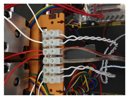
Put the red wire from the fan into one slot and the black wire into another. If you have a duo, put both red wires into one slot and both black wires into another.
