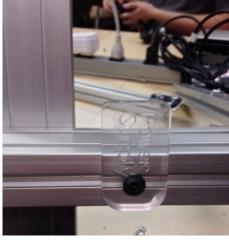
get it into the slot and flat). It is also a little hard to get it to catch- you may need to hold the nut in the track with another screwdriver again. You will adjust this significantly at the very end of the build- we are just putting it in a safe place for now. If you have a 1.5 inch thick power supply, you will skip this step.
