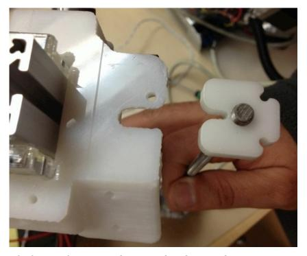
Insert the rod into the Z coupler tube and seat it on the shaft of the motor. Attach the top of the rod into the 3D printed end stop. Add M3 screws on top plastic part- be sure the slot on the small delrin nut is lined up with the internal protrusion inside the hole in the x end (see photo). Repeat on the other side. Notice that the X carriage has to be lifted to get these on, but you should be able to do this without taking off the X ends. It's awkward to get the nut on- put it on the tip
