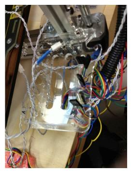
Run wires through the holes on the connector board mount as shown in the diagram on the previous page and clip connectors from the various components into place on the Azteeg board carefully. The board has labels, too.
