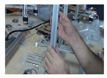
Push it into the slot to form the tape around the slider rail. Be sure that the tape is on tightly enough so that the tape makes nice right angles where it covers the protrusions.
