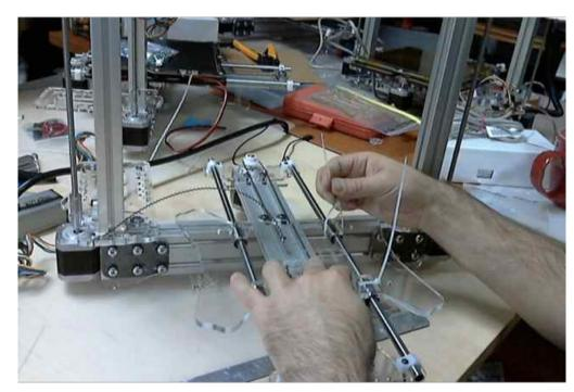
Take two zip ties and zip tie down just the left-side bearings. (Leave the right side for now so that you can have some access.) Be sure that you have not crossed over the synchromesh under the platform.
