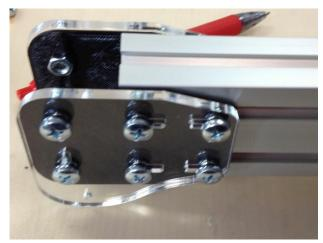
Then, attach ONLY the FIRST side beam. You can use what will be the top as a stop to guide how far down to push it. The bottom of the center aluminum rails should be flush with the bottom of the side rails.
