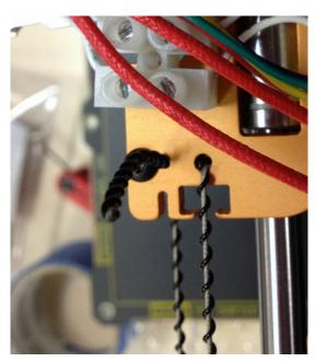
Thread synchromesh through holes in the x carriage and crimp down the end with screws from synchromesh kit. The synchromesh should go DOWN through the circular hole, then come UP through the slot with the screw. Tuck the excess into the slot on the side of the extruder carriage, or cut it off. If you cut it be sure to leave at least 25mm in case you need to reassemble the machine later.
