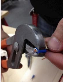
Crimp connectors on six of the ends (leave one set with just stripped wires at one end.)
