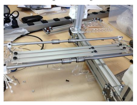
Insert the rods into the housing loosely on either end of the Y nylon end clamps. Be sure the clamps are loose so the rail will go in. Once the rods are in tighten the screws. The nylon should touch the acrylic once the screws are fully tightened.
