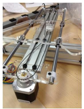
Take one of the motors and attach it to the end of the Y axis on the back of the machine using the M3 12 mm screws left over in the Y ends kit. You might have to loosen some of the other screws to align things; tighen all when the motor is on. The wires should face inward, (toward the front of the machine, toward the top of this picture). Place the synchromesh pulley (white) on top of the motor shaft. Pulleys go in such that the "brim" (wider part) is nearer the motor.
