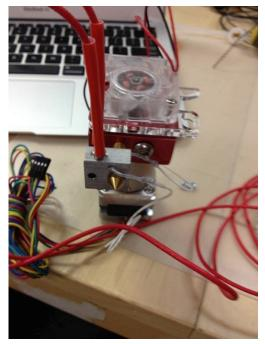
After you have attached the fan, then insert the heavy red wires with connectors on one end (the "heater cartridge") into the heater block as shown.
