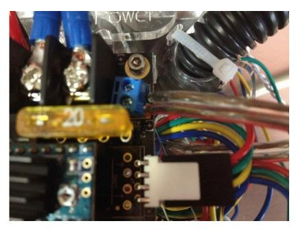
Attach the fan wires (be careful to hook up the red end to +) to the small blue screw-in connector box labeled "aux." (It is on the upper right of this picture, just below the screw in the corner of the board.)
