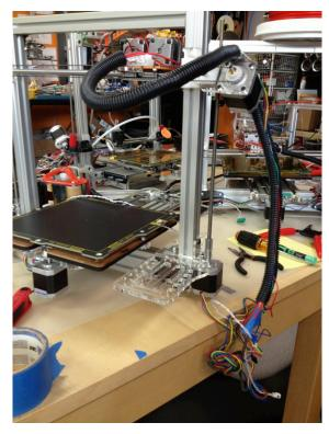
Run the wire bundle through the hole in the motor mount on the left X end and put on the conduit tubing. Make sure that the carriage can move end to end.
