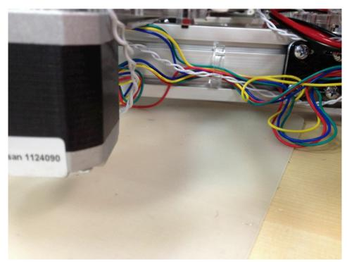
Tidy up the cables under the machine with the clear clips.
