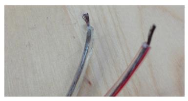
Take the 22 gauge wire and strip the ends. Split one end as shown for two or three inches. Connect the red end to the red fan wires, and the black end to the black fan wires. (The fan wires have a polarity.) We suggest (in the case of a duo) putting the thermistors on either end, and the shared (fan) connectors in the middle. The extruders are on the top of this picture. The connections coming out will go to the main electronics board.
