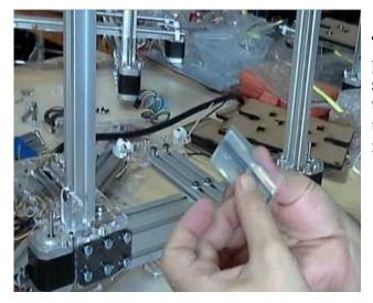
Take the rail slider and center the tape on the protruding central rail, which will fit into the slide. This tape is not meant to hold anything together; think of it as a lubricant that you are using to make the acrylic piece slide smoothly in the aluminum track
