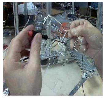
Take the part engraved "Y adj", and insert it into the Y carriage so that the protruding slotted cable guide part is to the front of the Y carriage. This set of pieces will allow you to adjust the tension on the Y axis synchromesh. There is a diagram on the platform for you to follow.
