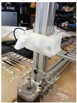
points down and will be the trigger for the Z end stop.
