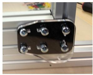
Attach the T-nuts to the Y center beam. The screw heads and washer should be on the top (grooved) side. The T-nuts should be on the bottom. The T-nuts will just catch on the first thread or so. Slide the Y beam onto the bottom beam. The inside of the side beam should be 13.5 cm from the side of the Y beam to center it. Tighten it down.
