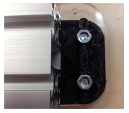
Put the nuts loosely on each screw and slide the first four nuts of each piece into the tracks of the aluminum bar that will be the bottom of the Bukobot. Repeat for the four brackets. Protruding acrylic feet should point down (away from the single-slotted part of the bottom frame.)
