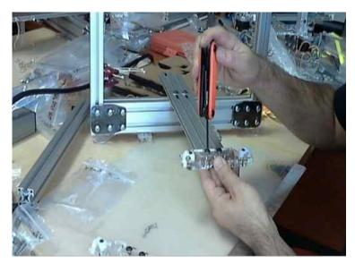
Attach the assembled ends to either side of the Y center beam. You have two screws left over that will be used later to attach the motor. Set them aside. You can put the small delrin (white) nuts on the ends now, but you will probably have to take at least one on each end off later on to put on the Y rods. For safekeeping put them on loosely now.
