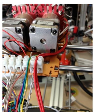
Now tidy up the wiring; run the wires under the extruders and tuck the heater wires in-between the top terminals so that things will not catch on the sides when the platform moves. Make sure no connections are loose and no wire strands are exposed.
