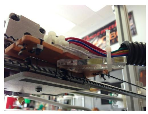
Add the strain relief piece of acrylic under the platform. It's shown here how it will look when the whole machine is done, just to orient you on what it is for.
