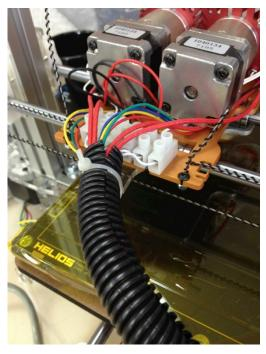
Use cable ties to tidy up the loose wires. There are strategic holes in the frame to accommodate the cable ties. For the wires coming off the X carriage, attach the cable conduit to the plastic strain-relief piece as shown.
