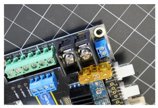
Take one black and red wire pair that has a connector crimped on both ends. Attach the red wire to the "+" connector with the big screw on the Azteeg board and the black one to the other one. (Large screws on top of this picture.)
