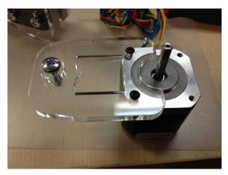
Attach a motor to each one as shown (this is the right-hand motor). Then slide them down the Z (vertical) rails on each side with the motors on the outside.
