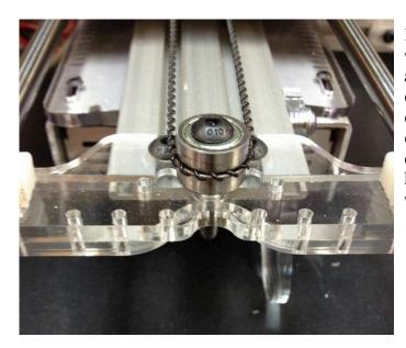
Put together another screw assembly with washer/bearing/washer/ bearing and attach it to the end of the Y carriage away from the azteeg board carrier (i.e., at the front of the Y carriage). It should be tight, but not enough to break anything. It's shown here with the synchromesh around it, which you will do in a minute.
