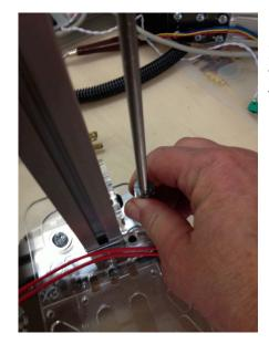
Next we will put on the top beam to finish the frame. First though you will need to lower the carriage by twisting the vinyl tube couplers over the Z screws on both sides.
