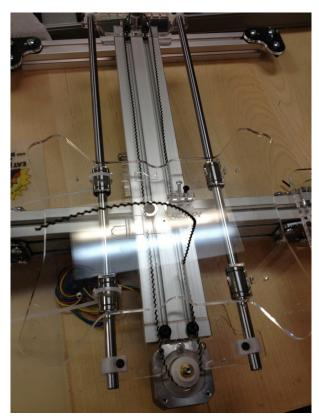
Take the Y-carriage acrylic piece; the "front" marking is away from the azteeg board mount. Run the synchromesh cable through the back of the board and through the pulley on one end of the y carriage and the roller on the other end. Attach the other end on the middle of the platform by pushing a screw into the provided hole as you did on the other loose end. Pull the synchromesh to make it tensioned but not extremely tight. There can be a little play in the synchromesh, but only a little.
