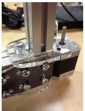
Another view of the assembled right hand side (as seen from the front.) Be sure that the motors are tight against the side of the frame and that there is no play anywhere in this assembly.
