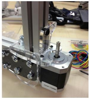
Attach the horizontal portion to the bottom track with a screw, then a washer, and then the acrylic spacer on the inside of the Z bar.
