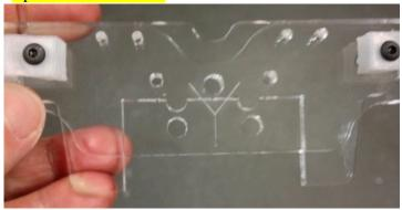
Assemble the Y ends (acrylic, says "Y" on the part) together with the white clips and M3 29 mm screws and nuts. Repeat for the second assembly.
