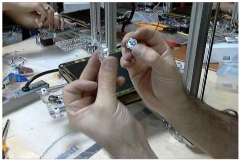
Put a spring in between the heated platform assembly (on the cardboard side) and the wood board on each of the three screws. Place the heated platform with the cable on the side nearest the Azteeg board (on the left, looking at the machine from the front.)
