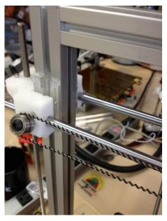
When that is done loosen the motor holder and swing it down which should add some tension. If it's too much, loosen slightly by loosening the tiedown screw. Cut off excess synchromesh once tension is correct.
