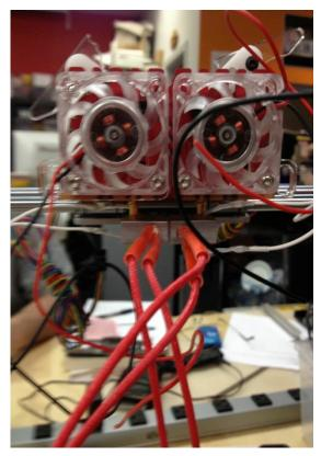
Then mount the extruder(s) onto the mount on top of the bearings as shown. If you have a single extruder, it will be on the right as seen from the front (with the nozzle closer to the centerline). Duo is as shown.
