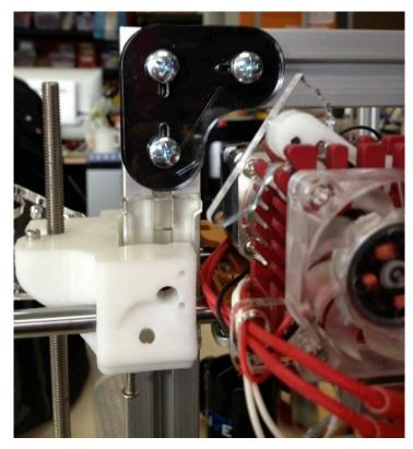
Be sure that the x ends (including the protruding acrylic sliders) are clear of the corner brackets. Check that the top is flush and there is no gap between sides and top. Tighten down the brackets.
