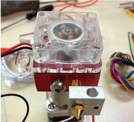
Next comes the fan spacer, and finally the fan. The fan label faces inward (will be hidden after assembly.)
