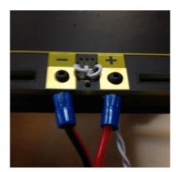
Take the red-black power wire pair that only has connectors crimped on one end. Connect the crimped end to the heated bed, with red wire going to +. Use the remaining M3 screws and nuts from the heated platform hookup kit. Attach the other end to the Azteeg board with red going to "H-bed +" and black to the other H-bed connection.
