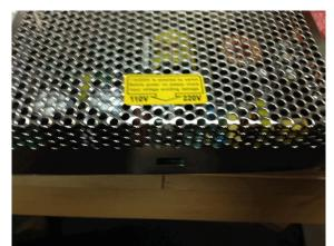
Pick up the power supply. Move the switch to 220 V or 110 (US), as appropriate.
