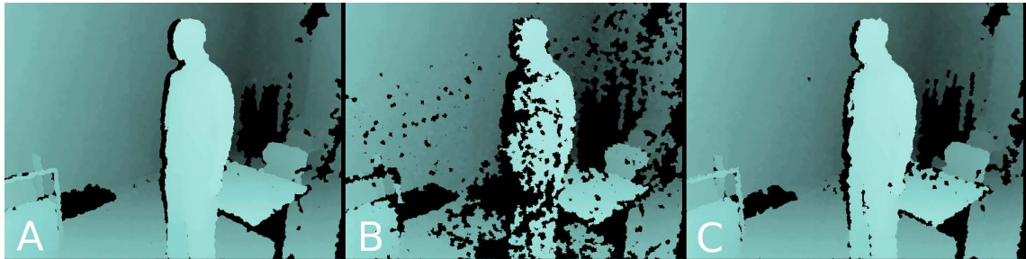
Figure 2.9: A - Depth map of room using a single Kinect. B - Depth map with 5 Kinect sensors overlapping the view, causing interferences and failures in estimation. C - Depth map with 5 overlapping Kinects while applying motion to every sensor. [MF12]
