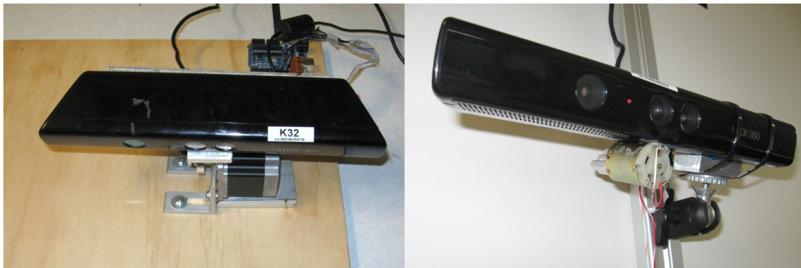
Figure 2.8: DC motor with eccentric mass attached to the Kinect for inducing vibration. [MF12]
