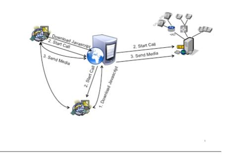
Figure 2: High level WEBRTC flow
