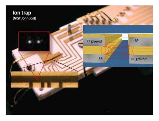
An ion trap is a combination of electric or magnetic fields used to capture charged particles in a vacuum. Ion traps have a number of scientific uses such as mass spectrometery, physics research, and controlling quantum states. The two most common types of ion trap are the Penning trap and the RF (Paul) trap (quadrupole ion trap).
