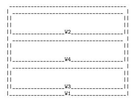
Now, when enlarging a window vertically, Emacs tries to obtain the corresponding space from its lower sibling, provided such a window exists. In our scenario, enlarging W4 will steal space from W3.
