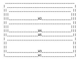
A new internal window W5 has been created; its children are W2 and the new live window W4. Now, W2 is the only sibling of W4, so enlarging W4 will try to shrink W2, leaving W3
