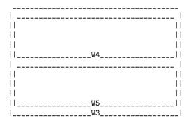
The split-window call has created a new live window, denoted by W5. It has also created a new internal window, denoted by W3, which becomes the root window and the parent of both W4 and W5.
