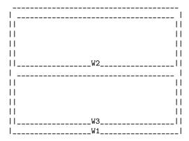
If window-combination-resize is nil, splitting window W3 leaves the size of W2 unchanged:
