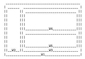
The root window of this frame is an internal window, W1. Its child windows form a horizontal combination, consisting of the live window W2 and the internal window W3. The child windows of W3 form a vertical combination, consisting of the live windows W4 and W5. Hence, the live windows in this window tree are W2, W4, and W5.
