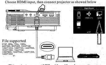
This projector support MHL cable and I-push connection. Detailed using method please refer to MHL and I-push user
